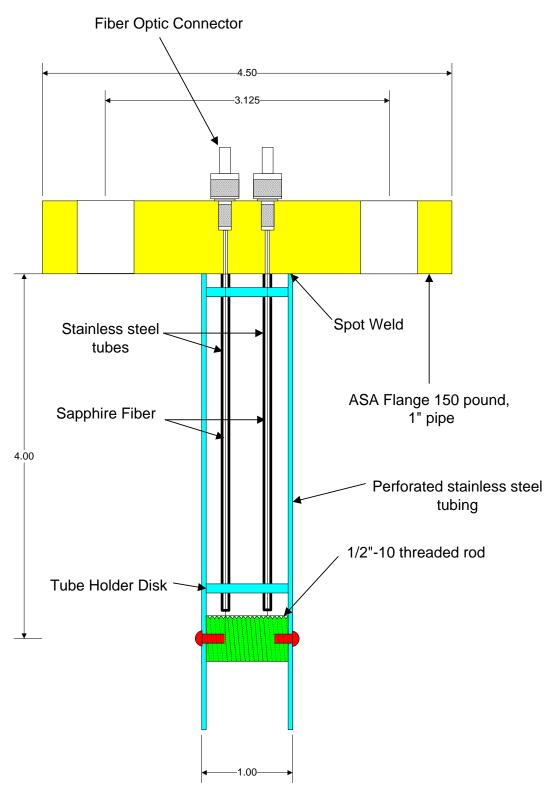
Thoughtventions developed the fabrication procedure for making this commercial fiberoptic chemical sensor. The problem was to wind 10 turns of 100 micron diameter sapphire fiber around a mandrel and then pot the fibers in standard connectors reliably, without breaking the fiber.
